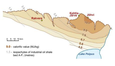
Figure 1. Thickness and calorific value of the oil shale seam in the oil shale deposit of Estonia
