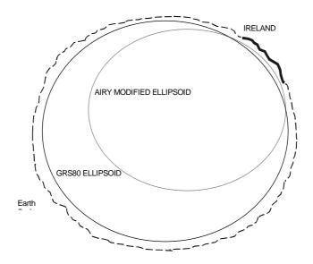
Diagram 5: Exaggerated diagram of ellipsoids and earth surface.
